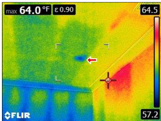
Thermal image of suspect leak
